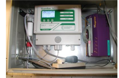
The device (Guardian®) allowing methane emissions measurements at the ACS
