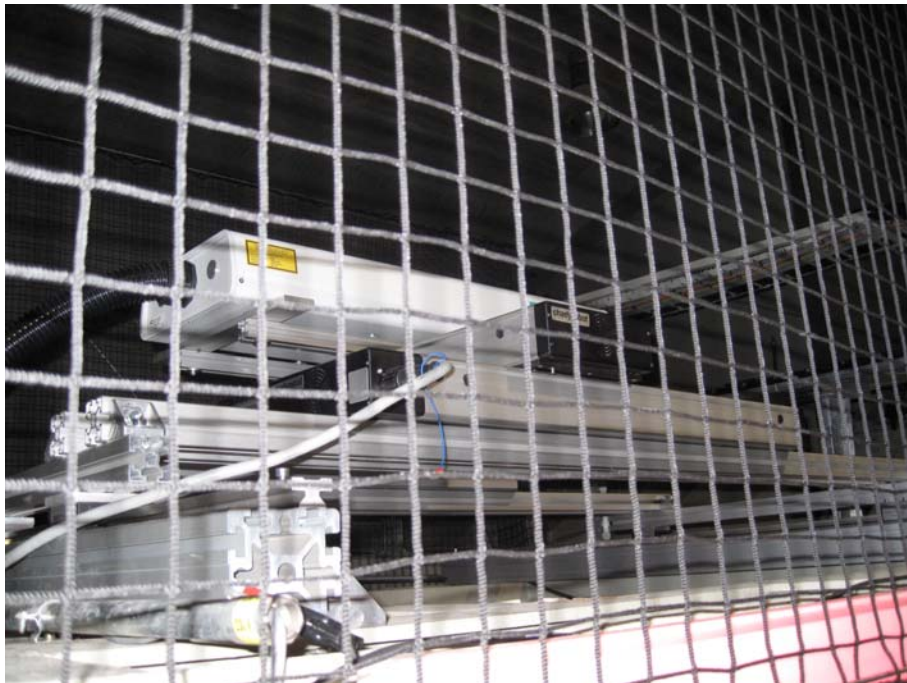
Laser on its translation system on the top of the test section
